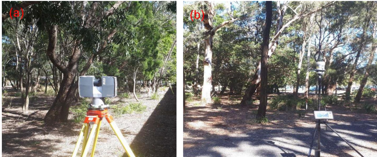
Figure 2. (a) The TLS data collection; and (b) RTK GNSS surveying.
